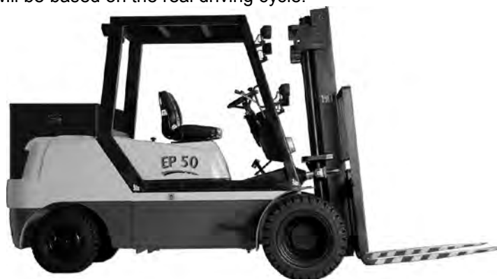
Fig. 1. The Project idea for hybrid fuel cell power system is based on a standard 2.5 or 3.5 tons battery forklift on the Balkancar Records manufacturer.
